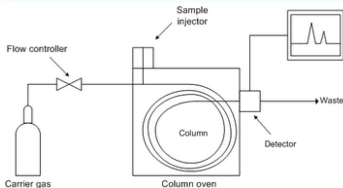
A gas chromatograph is a chemical analysis instrument for separating chemicals in a complex sample. A gas chromatograph uses a flow-through narrow tube known as the *column*, through which different chemical constituents of a sample pass in a gas stream (*carrier gas*, *mobile phase*) at different rates depending on their various chemical and physical properties and their interaction with a specific column filling, called the *stationary phase*.
