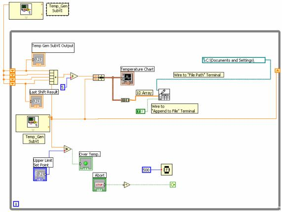
7. Type in the desired path in the PATH CONSTANT box. Note for this example the PATH BOX contains the following path:
